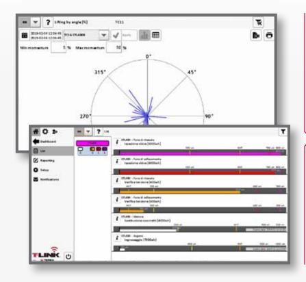
**T-Link** has 11 analytics templates and if not enough, you can use T-Link's configurable analytics engine to create your own combinations of 35 parameters. You can monitor parts wear and under which conditions the crane has been operating. Moreover, you can predict maintenance needs. Data can be visualized as charts or tables, printed or downloaded. If you run a rental business, T-Link analytics allows you to bill operational time
